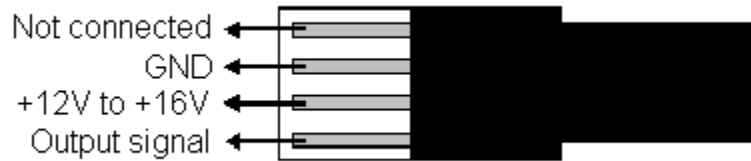
FIG. 1-4 MOLEX CONNECTOR PIN-OUT IN MT VERSION
